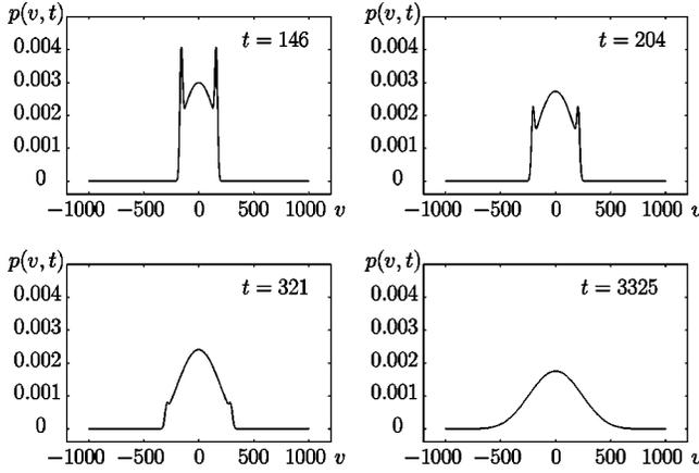
FIG. 2. Plots of  $p(v, t)$  resulting from a numerical integration. Parameters:  $\gamma = 10^{-3}$ ,  $\lambda = 0.02$ ,  $W = 1$ ,  $4T_V^* = 2000$ ,  $T_V = 1050$ . End points are at  $v = -1000$  and  $v = +1000$ .
