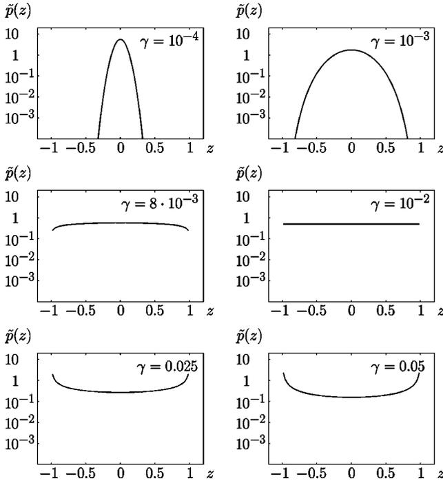
FIG. 1. Plots of Eq. (9) for different values of  $\gamma$ . The abscissa refers to the rescaled velocity  $z$ , the ordinate to the rescaled distribution  $\tilde{p}(z)$  in logarithmic scale. Parameters:  $W=1$ ,  $\lambda=0.02$ .
